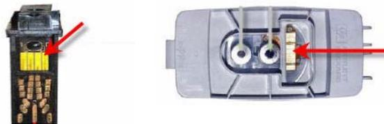
Ink must be purchased from MCS in order for this technology to be detected. The 4250 will not print without ink from MCS. If other ink is inserted into the device an error is displayed and the equipment does not function.
